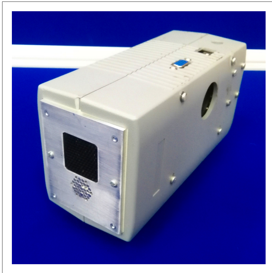
Figure 2. Close up of the ensoufflement device. At the front of the device the array of 31 microphones (Knowles FG series) can be seen. The Senscomp Series 7000 ultrasonic speaker is located above this array. DOI: 10.7554/eLife.14188.004
