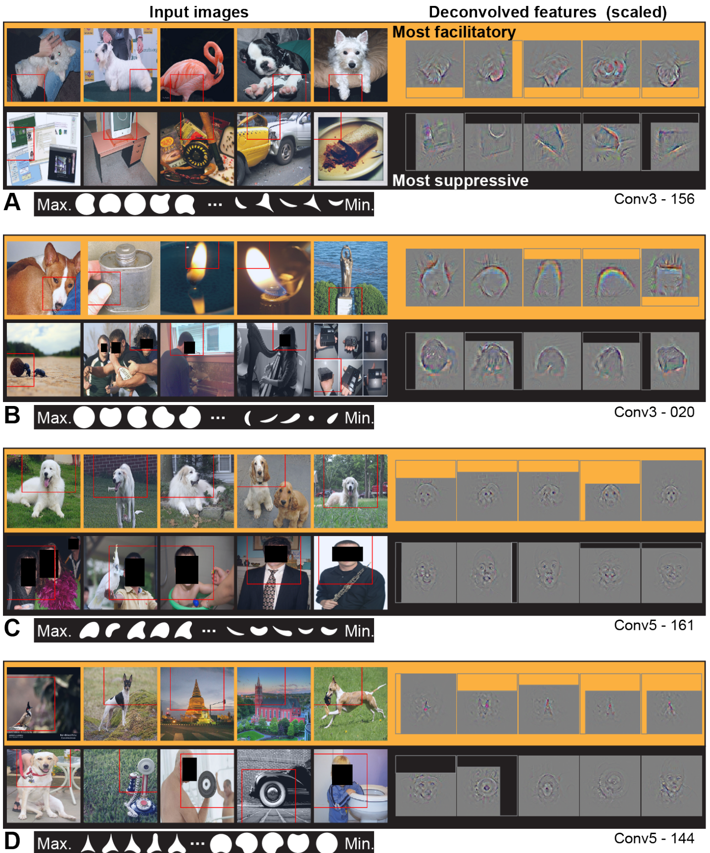
Figure 10. Visualization of APC-like units in layers Conv3 to Conv5. (A) Visualization for unit Conv3-156, using the same format as Figure 9. Deconvolved features are scaled by 1.8 for visibility. (B) Same as (A), for unit Conv3-020. (C) Same for unit Conv5-161, but deconvolved features are scaled by 1.15. (D) Same as (C), but for unit Conv5-144. For APC fit parameters, see Table 1 in main text. The un-redacted input image thumbnails were accessed via the ImageNet database and the original image URLs can be found through this site ( http://image-net.org/about-overview ). These thumbnails may be subject to copyright. They are not available under CC-BY and are exempt from the CC-BY 4.0 license.
